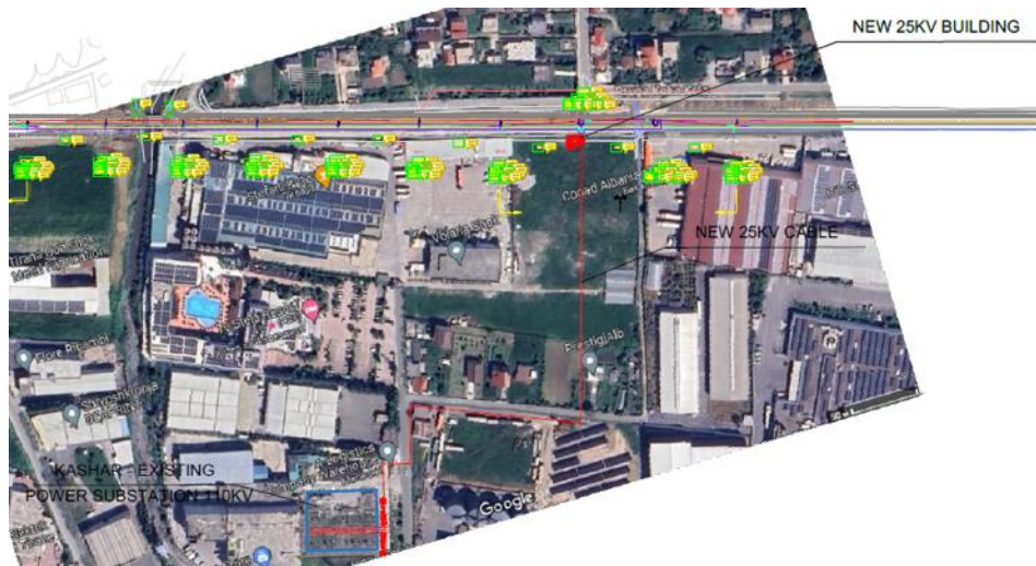
Figure 9 Alternative 2 New transformer 110kV/25kV inside the boundaries of existing power substation KASHAR and new 25kV facility near the railroad
