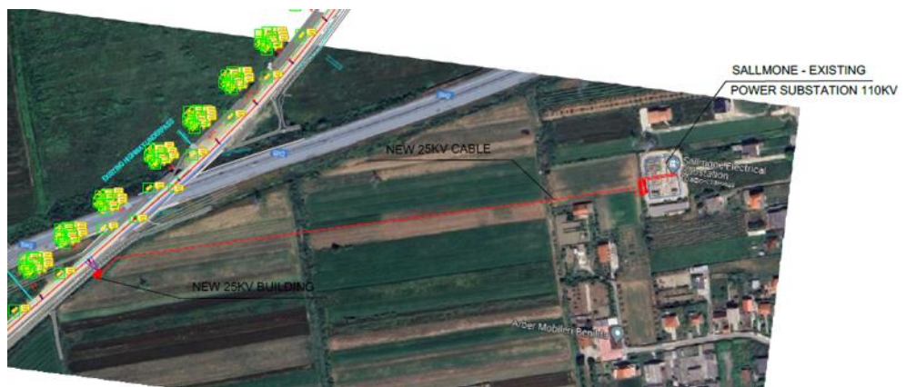
Figure 10 Alternative 2 New transformer 110kV/25kV inside the boundaries of existing power substation Sallmone and new 25kV facility near the railroad
