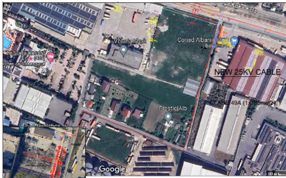
Figure 7 Alternative 1 New transformer 110kV/25kV and new 25kV inside the boundaries of existing power substation Kashar
