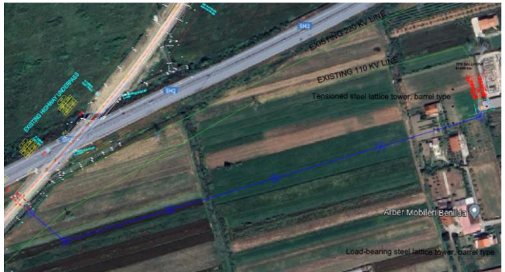
Figure 8 Alternative 1 New transformer 110kV/25kV and new 25kV next to existing power substation Sallmone
