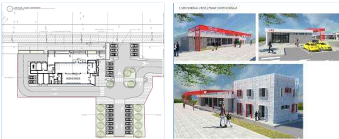
Figure 3: General layout and 3-D view of Lac station
